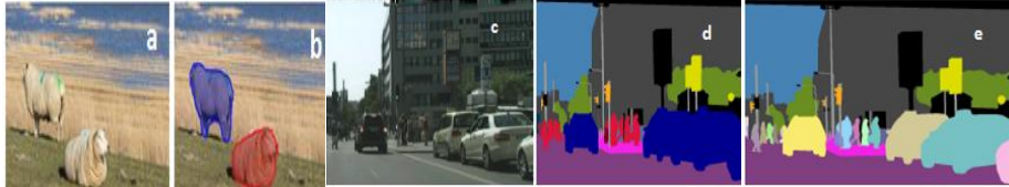
Fig 2: (a) image (b) after applying Instance segmentation [2] (c) image (d) after applying semantic segmentation [14] (e) after applying panoptic segmentation [15]
