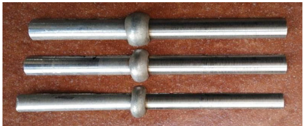
Fig. 1 Dissimilar weld joints
