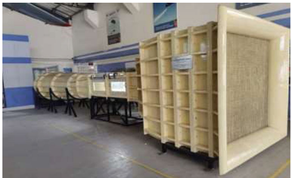
Fig. 2 Low-speed subsonic wind tunnel facility (HITSLSWT)
