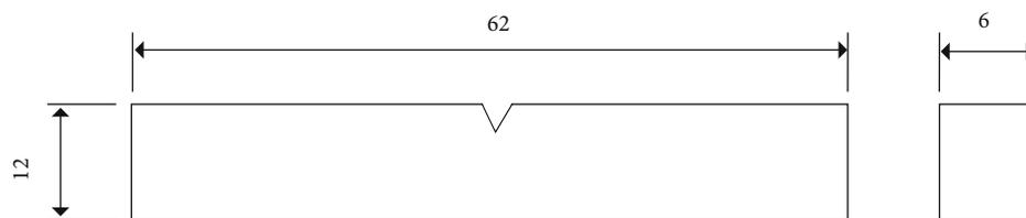
FIGURE 6: Schematic diagram of impact test specimen.
