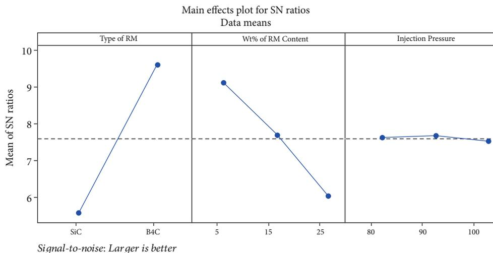
FIGURE 9: Effect of control factors on impact strength nylon 66 composites. Optimum levels: type of RM = B<sub>4</sub>C; wt% of RM content = 5%; Inj. pressure = 90 MPa.
