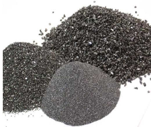
FIGURE 2: Boron carbide.
