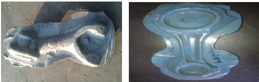
Fig 08 Flash Formation Around Job.
